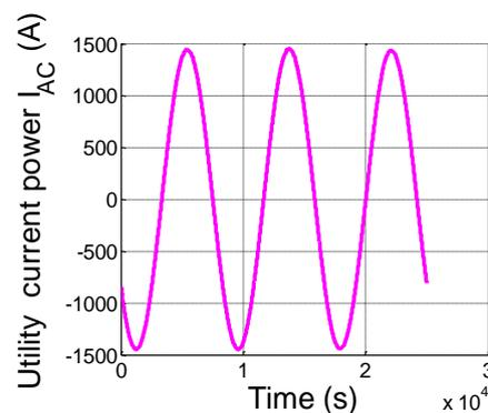
**Figure 12.** Simulation results on utility power current in grid connected hybrid PV/WT system
