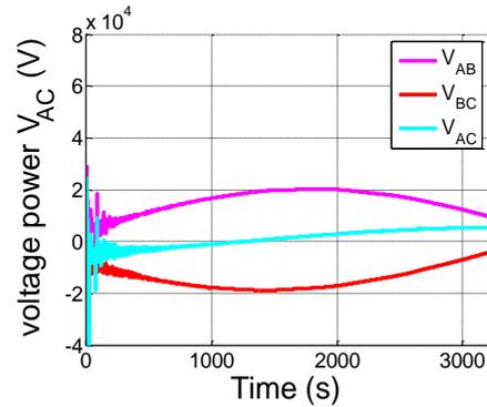
**Figure 10.** Simulation results of power voltage in grid connected hybrid PV/WT system
