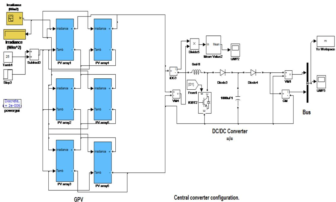
Figure 4. MATLAB/Simulink diagram for the central converter configuration
