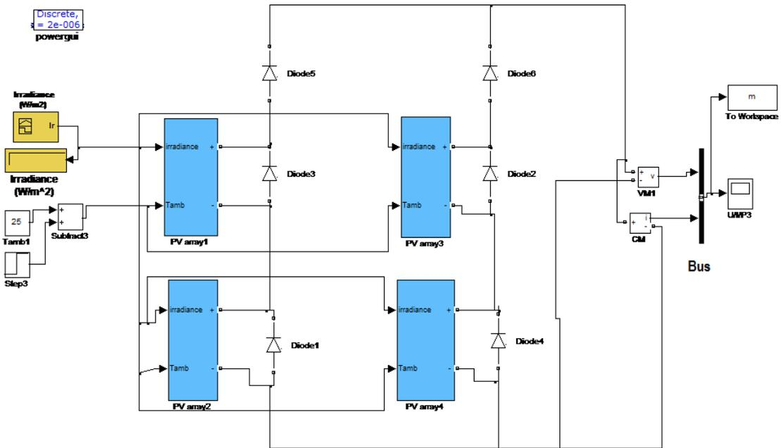
Figure 3. MATLAB/Simulink diagram for the connection of PV modules
