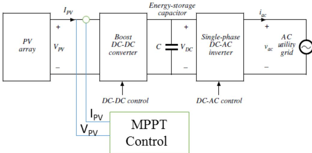
Figure 1. Control scheme of the grid connected system PV by using the MPPT
