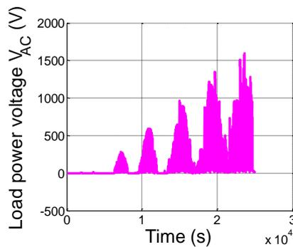
**Figure 14.** Simulation results of grid load power voltage
