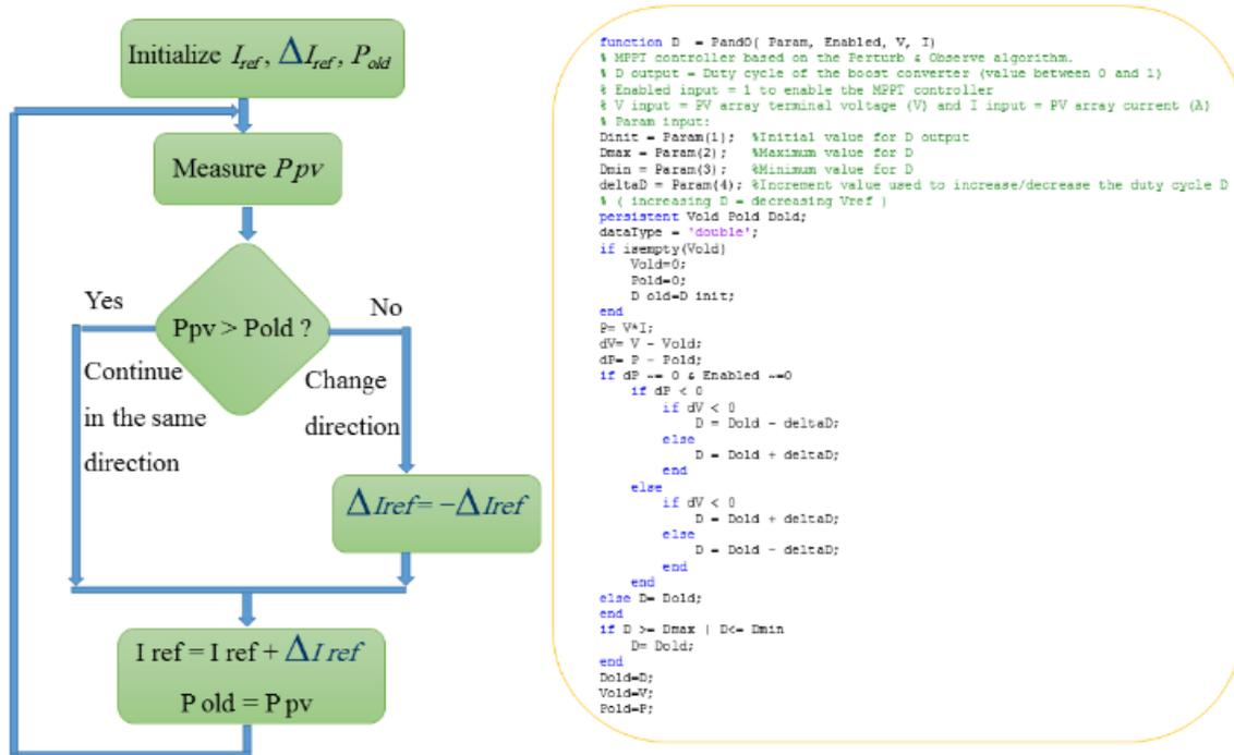
Figure 2. Initiating the MPP tracking algorithm in our study
