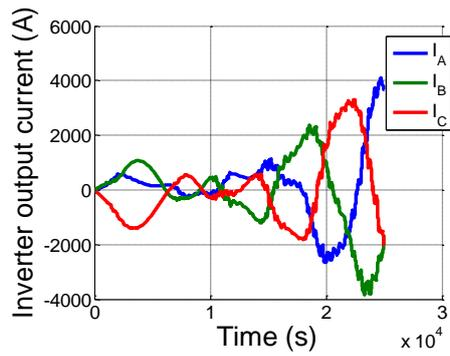
**Figure 9.** Simulation results of AC Inverter output power current
