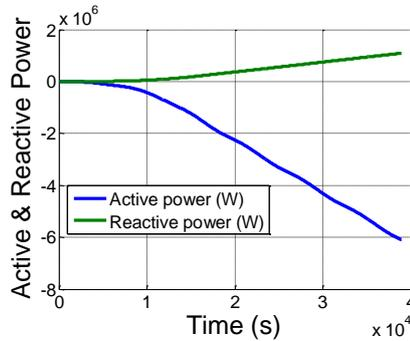
**Figure13.** Simulation results of active and reactive power distribution in grid connected hybrid PV/Wind turbine system
