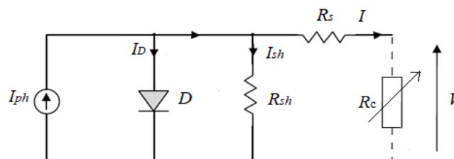
Figure 2. Modeling of a photovoltaic cell
