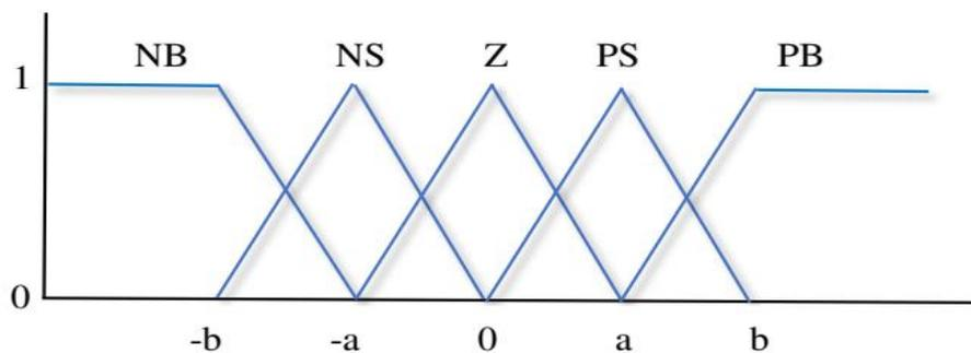
Figure 9. Fuzzy membership functions used in the fuzzification process
