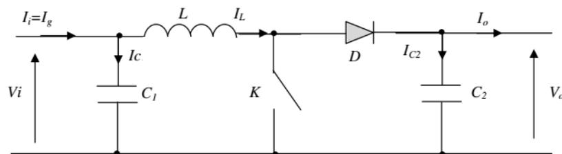
**Figure 4.** Circuit of boost-converter
