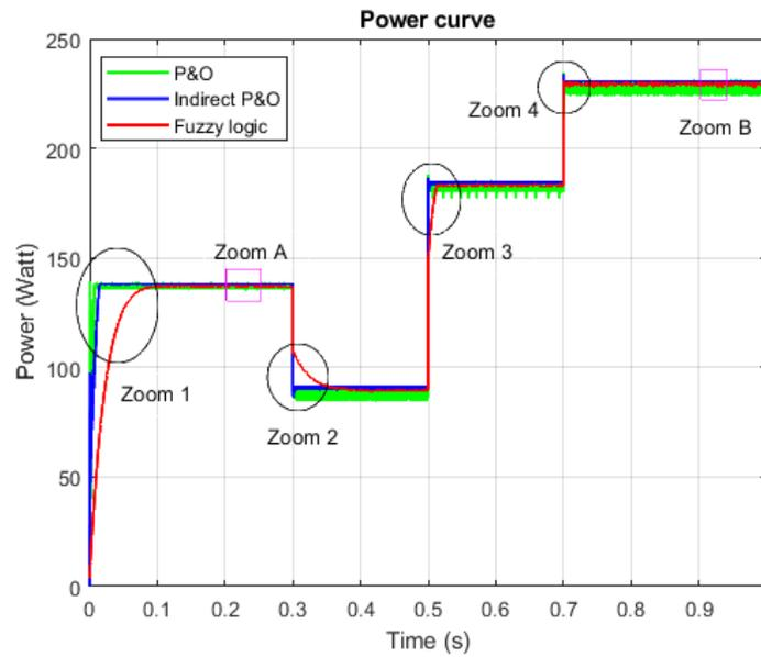
**Figure 14.** (a) Power curves of different methods under temperature (25 °C) and varying irradiance
