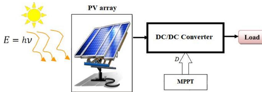
Figure 1. Block diagram of PV system
