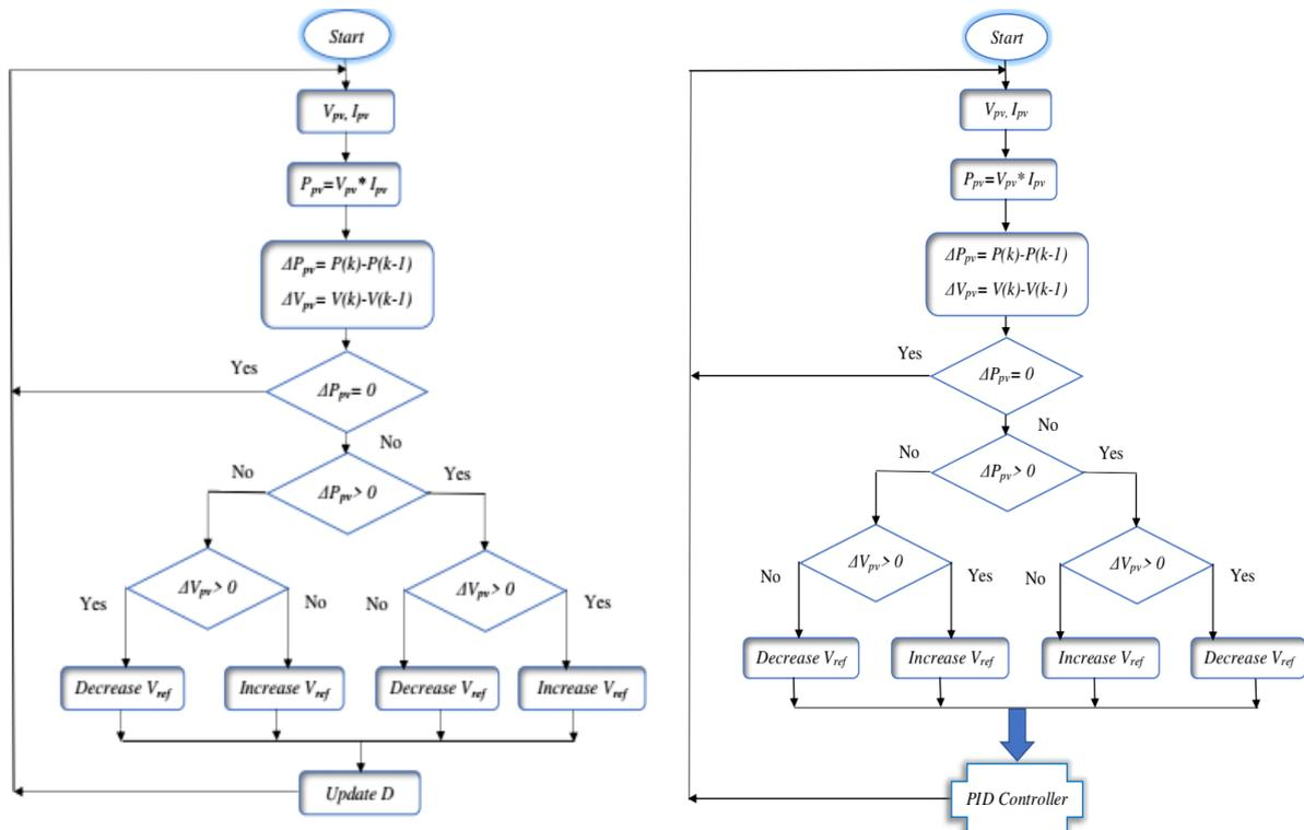
Figure 7. Flowcharts of P&O and indirect P&O algorithm respectively
