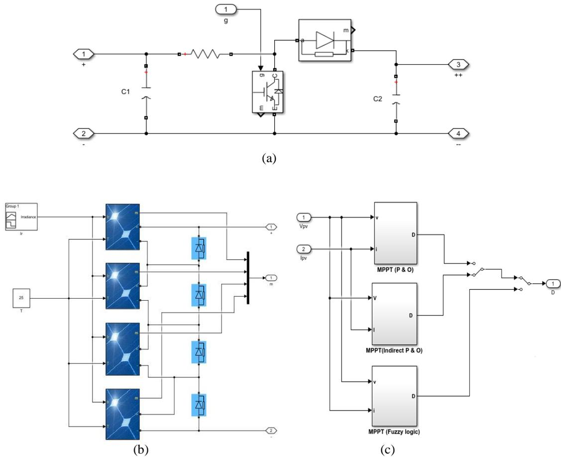
**Figure 11.** (a) DC/DC converter (Boost), (b) Bloc of PV array, (c) Choice of MPPT technique
