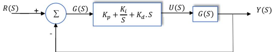
Figure 6. Block Diagram of the PID Controller
