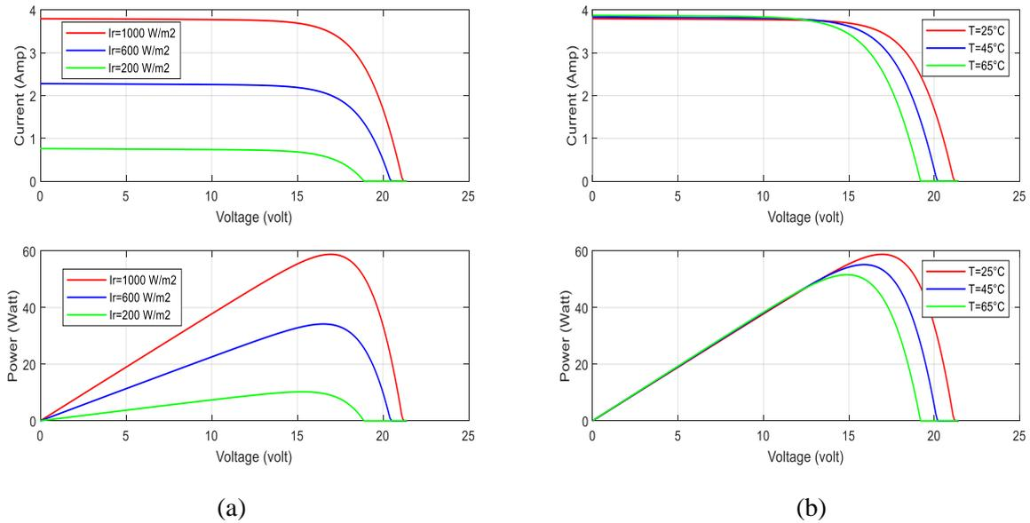
**Figure 3.** Characteristics of Solar panel for different irradiance and temperature values
