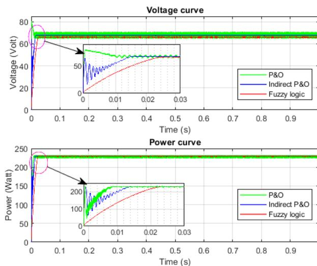
**Figure 12.a.** Voltage and Power curves of different algorithms under uniform irradiance (1000W/m<sup>2</sup>) and temperature (25 °C)
