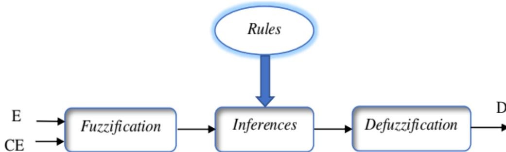
Figure 8. Block diagram of fuzzy logic control
