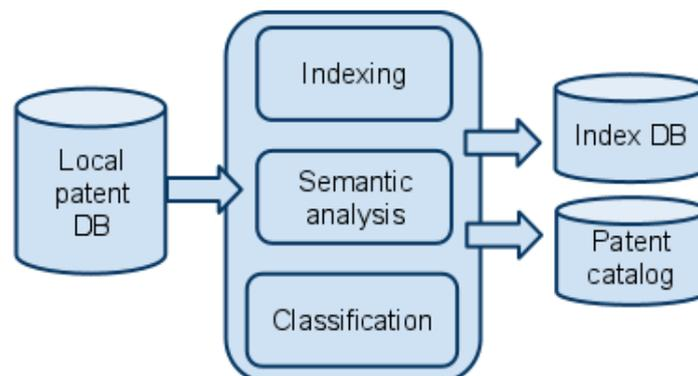
**Figure 3. The patent processing module**
