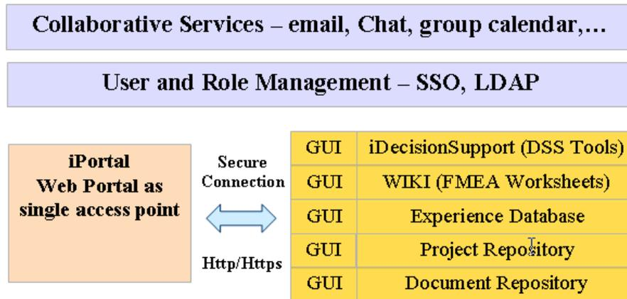
Figure 8. The components of idDesign platform
