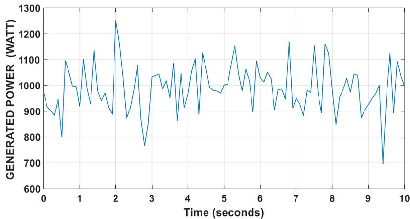
**Figure 7.** The generated electrical power  $P_{PV-w}$  from the PV-wind hybrid system
