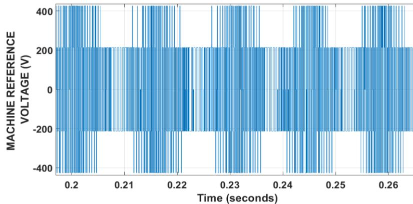
Figure 14. Machine stator voltage (phase 1)
