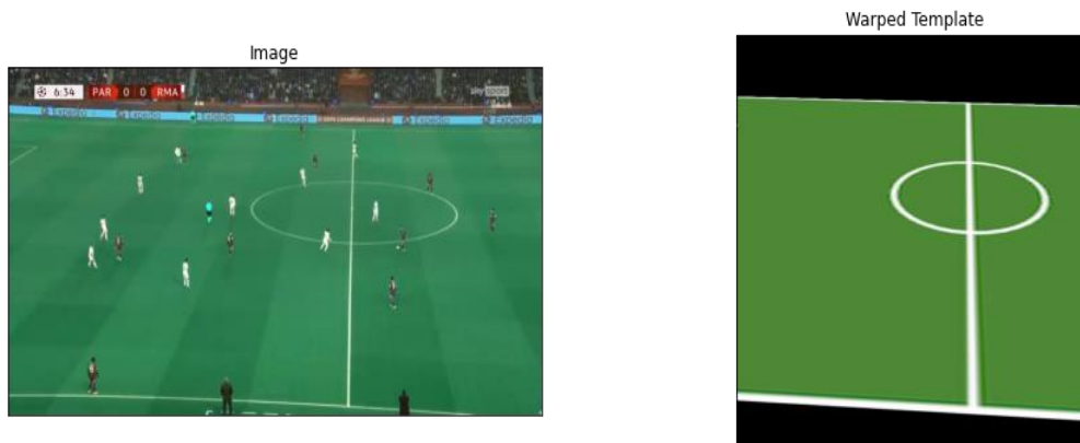
Figure 7. Warped Template from computed homography matrix
