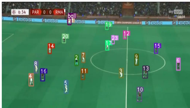
Figure 3. Example output image for player, ball and Team Tracking using DeepSORT and YOLOv5
