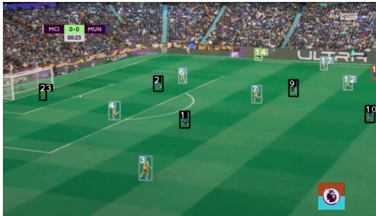
Figure 4. Boundary Box colored based on the team identified by the K-Means model
