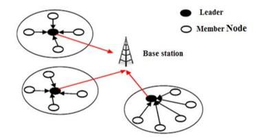
Figure 1. Simple model of clustering in wireless sensor network
