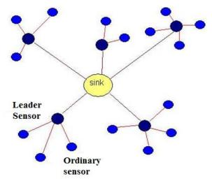
Figure 2. Clustering in wireless sensor networks
