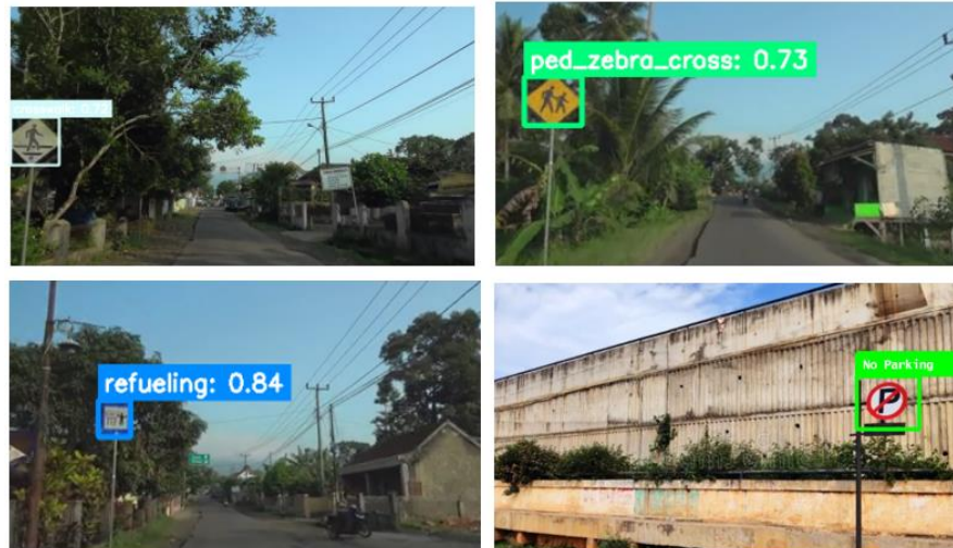
Figure 6. Example of detection outputs from the proposed environment-aware YOLO system, showing traffic signs identified with bounding boxes, class labels, and confidence scores under diverse road conditions (Source: Authors' own work)
