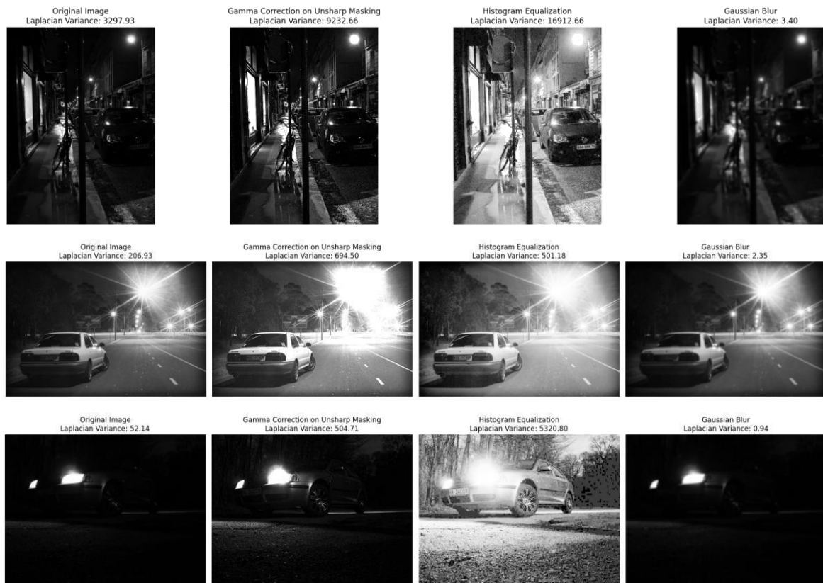
Figure 2. Vehicle license plate images in a low-light environment. Column 1: Input images; Column 2: Enhanced images using gamma correction on unsharp masking; Column 3: Enhanced images using Histogram equalization; Column 4: Enhanced images using Gaussian blur
