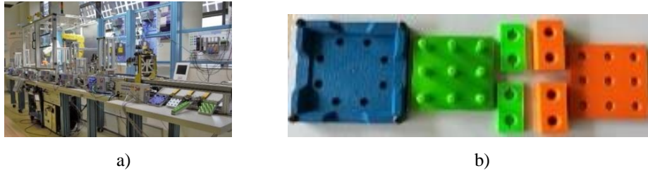
Figure 1. a) The flexible manufacturing system from ICSTM; b) The product components used to produce the finished products in the manufacturing system
