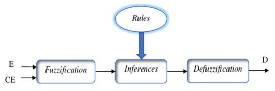
Figure 8. Block diagram of fuzzy logic control
