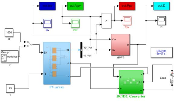
Figure 10. Simulink model for global PV system
