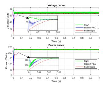
Figure 12.a. Voltage and Power curves of different algorithms under uniform irradiance (1000W/m<sup>2</sup>) and temperature (25 °C)
