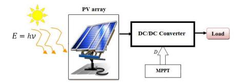
Figure 1. Block diagram of PV system
