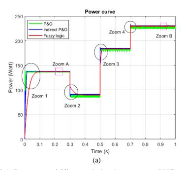
Figure 14. (a) Power curves of different methods under temperature (25 °C) and varying irradiance
