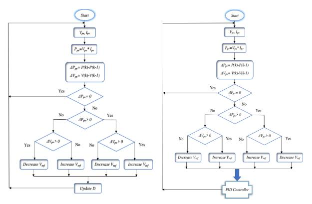
Figure 7. Flowcharts of P&O and indirect P&O algorithm respectively
