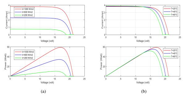
Figure 3. Characteristics of Solar panel for different irradiance and temperature values
